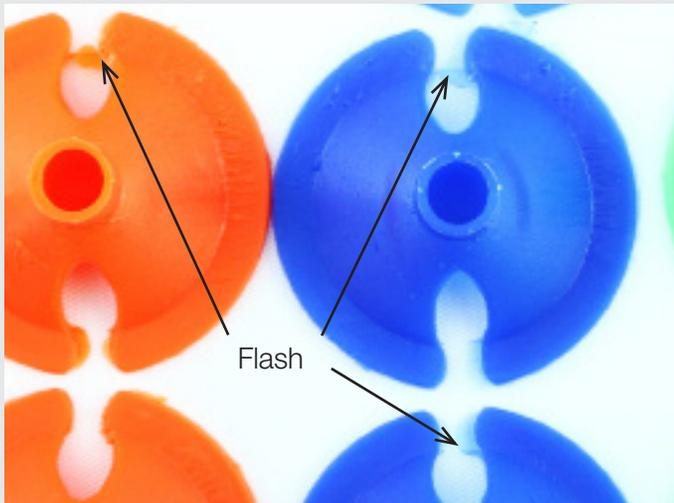
Unightly flash remains on parts produced by injection molding.
