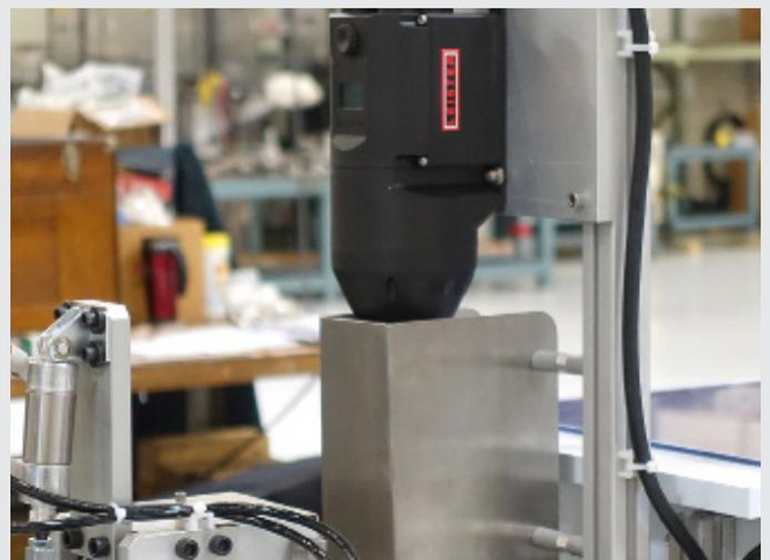
Leister MISTRAL hot-air blower installed in a production system.
