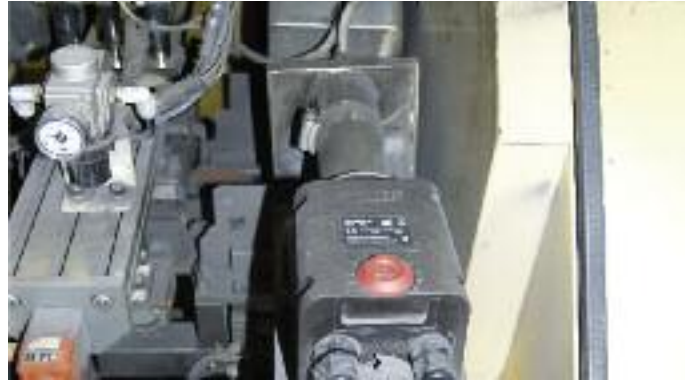
Deflashing foil sleeves from charcoal filter elements with an LHS 40L air heater.
