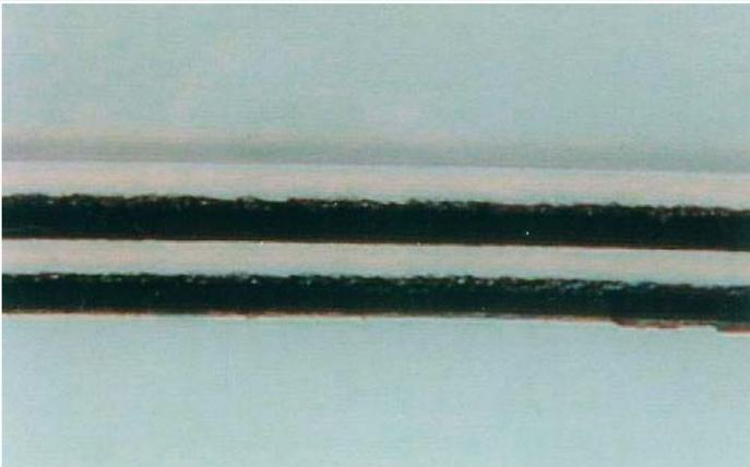
*Above: cross-section of a TPO-sheet with standard nozzle (sevenfold enlargement).*
