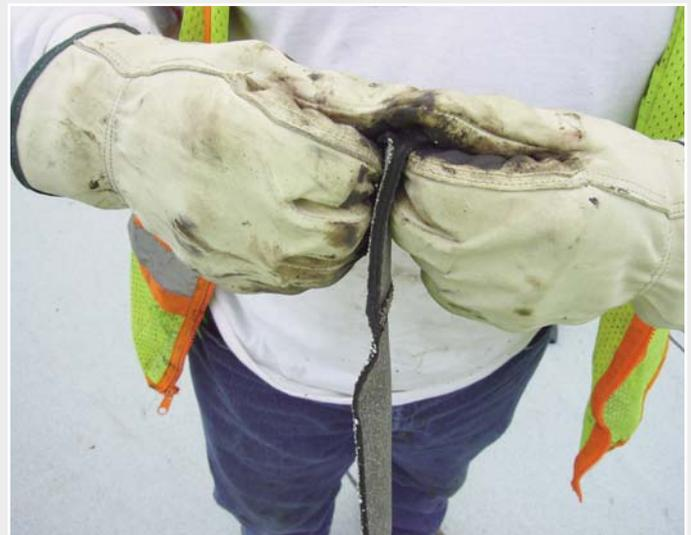
*The peel test demonstrates that the weld seam strength is significantly better with the BITUMAT B2 than with a naked flame.*
