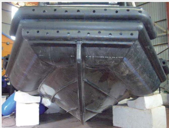
*Boat underside with blunt-welded and extruded parts*
