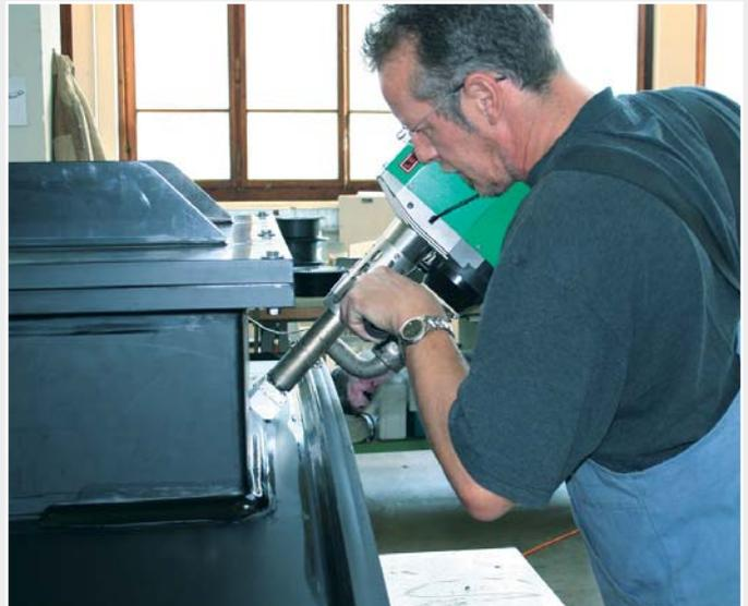
*Extrusion joining the inspection hatch on to the bowed PE wall element using a WELDPLAST S.4 .*
