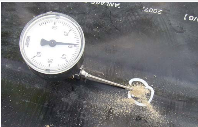
The injector needle is used to check the integrity of the (perfectly) welded seam.
