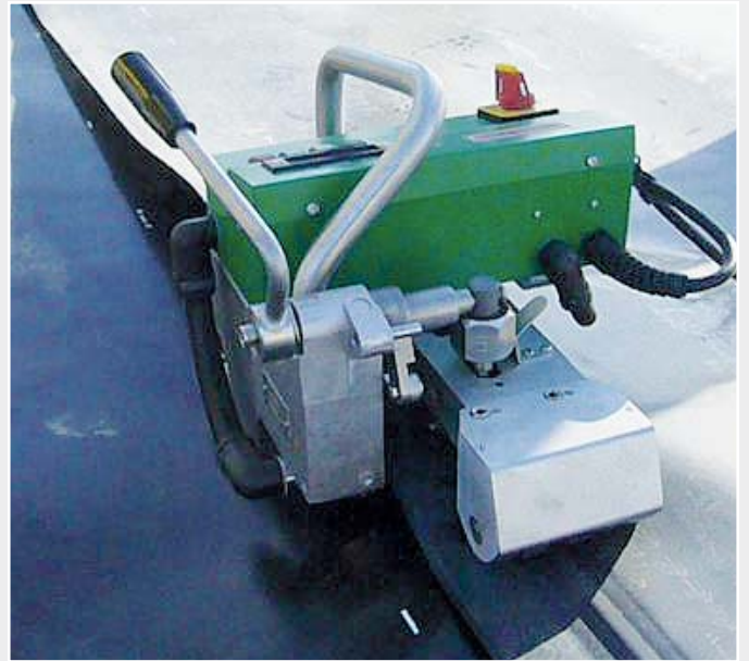
The ASTRO welds the HD-PE sealing tracks at a speed of up to 5 m/min.
