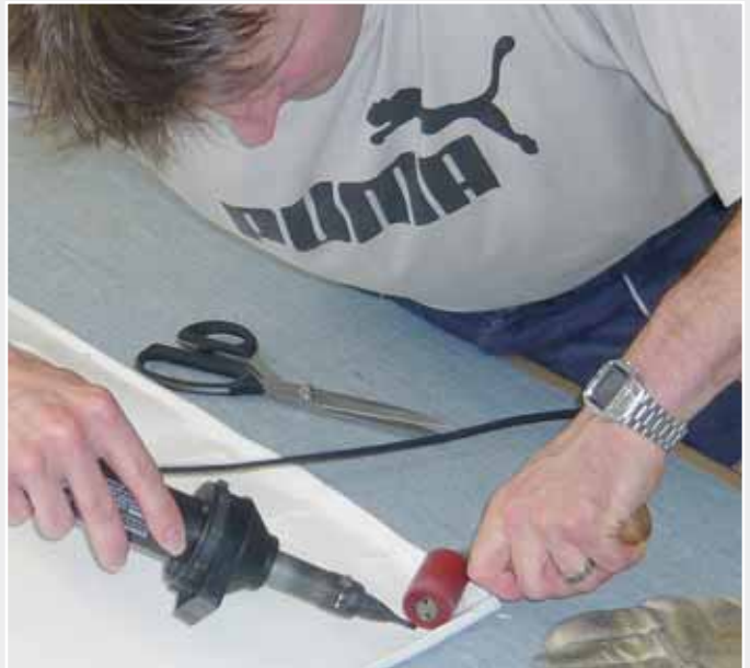
The HOT JET S from Leister is a handy help for details.
