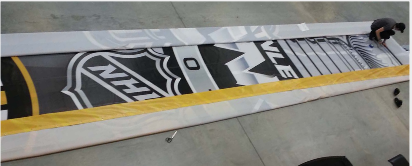
Most of the banners were 150 by 50 feet, and welded at the company's Strafford, New Hampshire production Facility.
