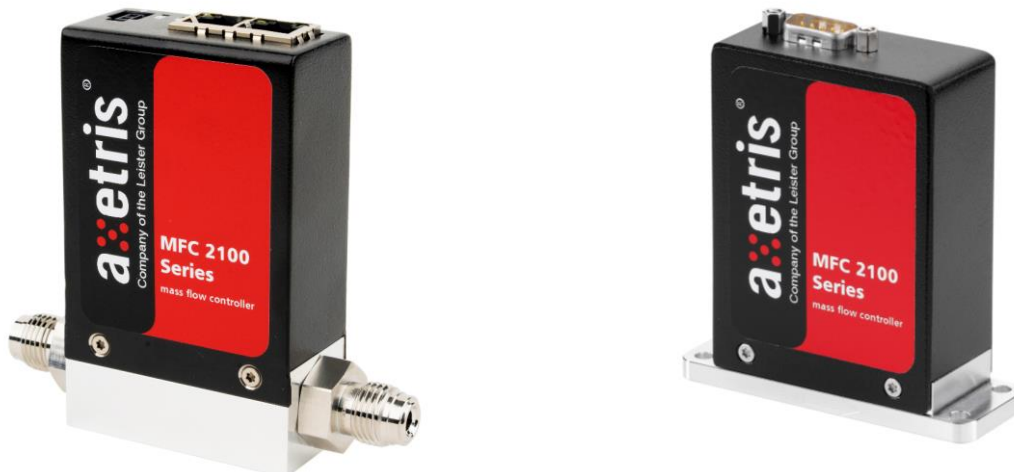
Figure 1 Mass Flow Meter MFM 2100 and Mass Flow Controller MFC 2100 series available with the following interfaces: RS-232 + analog 0...5V, RS-232 + 4...20 mA, RS-485 half duplex, RS-485 full duplex, PROFINET, EtherCAT. Left: MFC 2162 side port connector and RJ45, Right: MFC 2122 down port connector and D-Sub 9.
