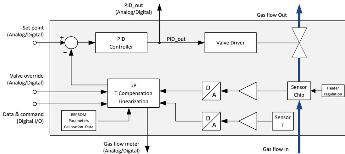
**Figure 2** Block diagram of the MFC 2100 and MFC 2200 series of mass flow controller
