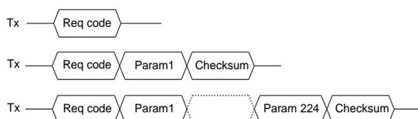
Each request begins with a one-character code identifying the request. If the request to be sent is coded on more than one byte, a checksum has to be added at the end of the command. The checksum is the sum of all the preceding bytes value, including the request byte, truncated to the last 8 bits of the results.
