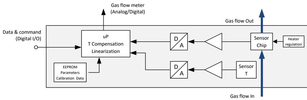
**Figure 1** Block diagram of the MFM 2100 and MFM 2200 series of mass flow meter
