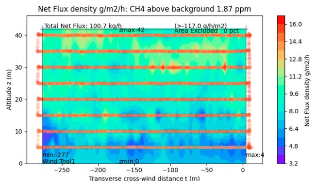
When determining emission rates from a source, the drone maps out a vertical data grid of gas concentrations and wind vectors. Based on the data, Explicit is able to calculate how much total CH<sub>4</sub> is being emitted (kg/h) to help quantify emissions and locate leak(s).
