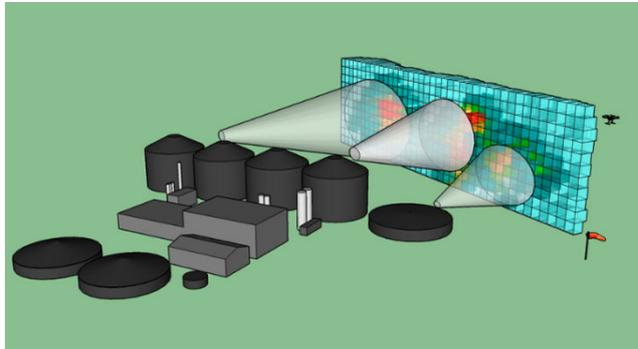
Mapping of CH<sub>4</sub> emissions measured at a biogas plant plant by using sniffer drones.
