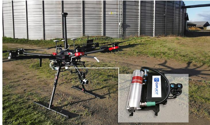
The LGD Compact integrated by Explicit ApS during first field test for monitoring CH<sub>4</sub> emissions from biogas plants.
